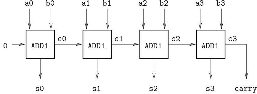
Figure 6: 4-bits adder
