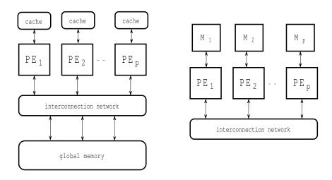
Figure 3: Shared and distributed memory multiprocessors
