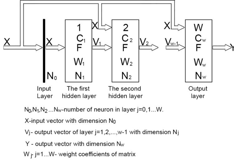
Figure 2: Structure of Cross Forward Connection ANN
