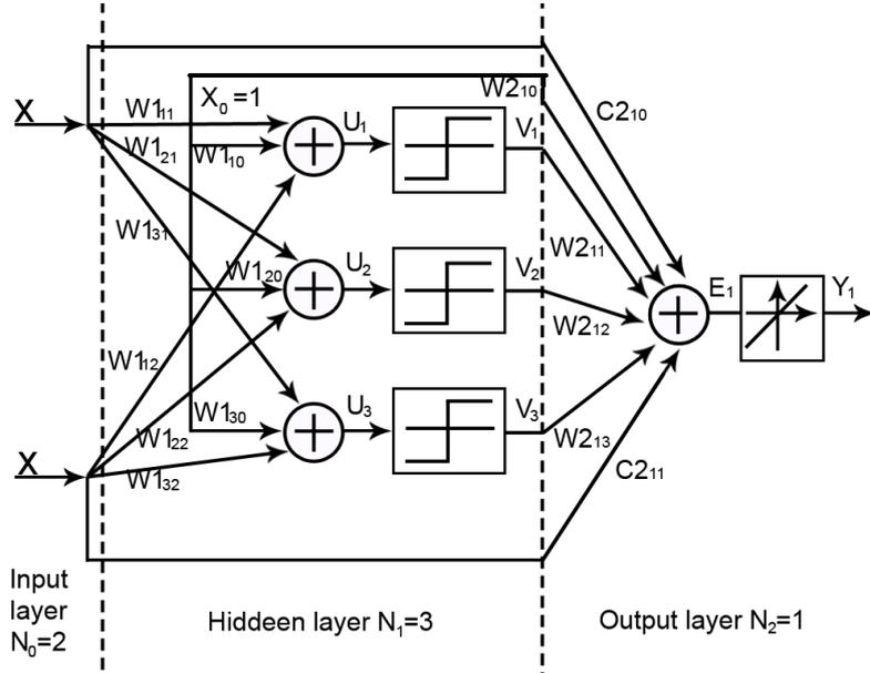
Figure 3: Two Layer ANN with Cross Forward Connection
