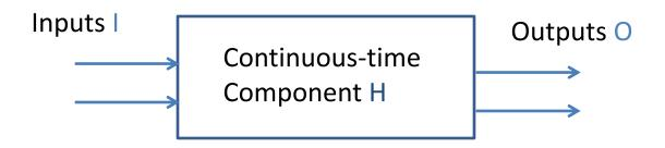
A continuous-time component H maps input signals I(t) to output signals O(t)
