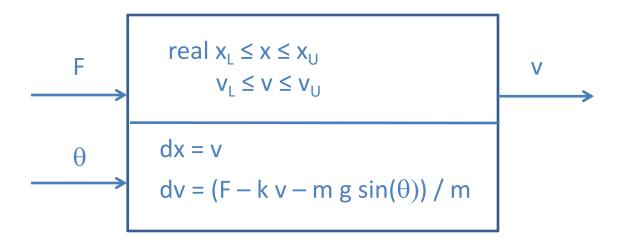
The road's slope, denoted by  $\theta$ , models disturbance, or an uncontrolled input
