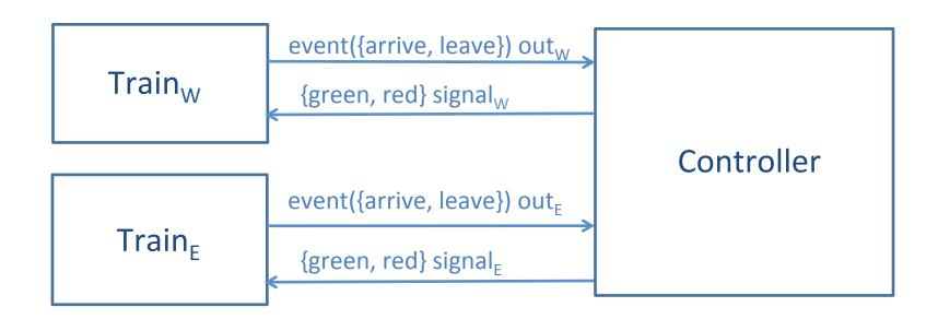
Safety Requirement: Trains should not be on bridge simultaneously Formally, the following should be an invariant:
