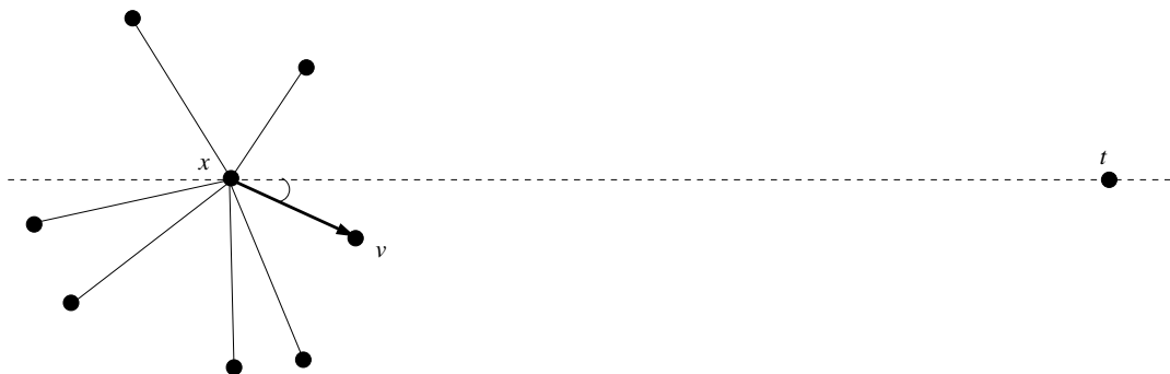
Figure 2: The node x , on receiving a message m , intended for the destination t , forwards m to a neighbor v that makes the smallest angle with \vec{xt} .
