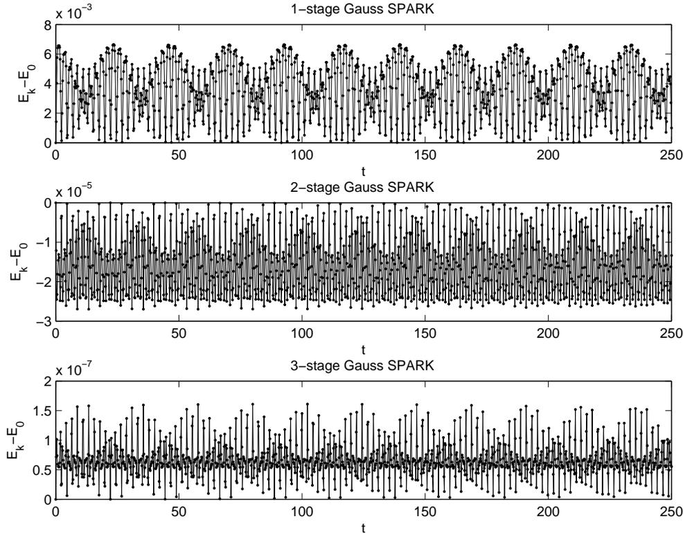
FIG. 8.1. Energy error of the  $s$ -stage Gauss SPARK methods for  $s = 1, 2, 3$  applied with constant stepsize  $h = 0.2$  on the interval  $[0, 250]$  to the nonholonomic particle.
