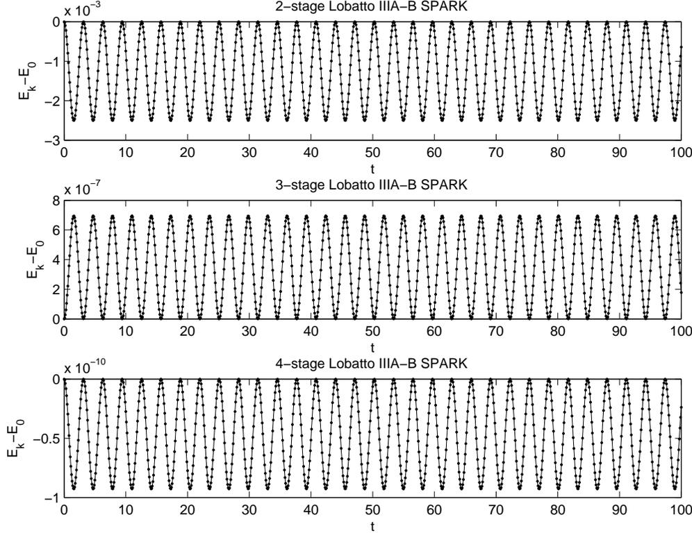
FIG. 8.2. Energy error of the  $s$ -stage Lobatto IIIA-B SPARK methods for  $s = 2, 3, 4$  applied with constant stepsize  $h = 0.1$  on the interval  $[0, 100]$  to the skate on an inclined plane.
