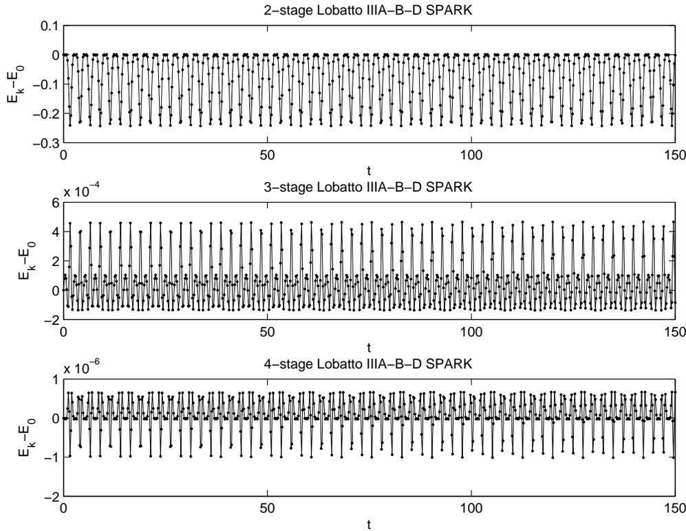
FIG. 8.3. Energy error of the  $s$ -stage Lobatto IIIA-B-D SPARK methods for  $s = 2, 3, 4$  applied with constant stepsize  $h = 0.2$  on the interval  $[0, 150]$  to the mobile robot with fixed orientation and a potential.
