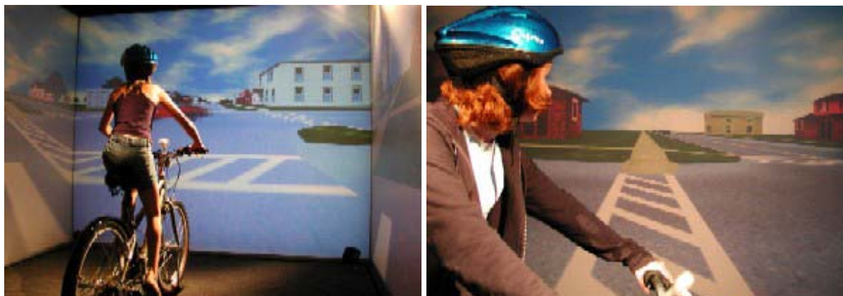
Figures 1a (left) and 1b (right). Photographs of the bicycling simulator. Note that the visual angles are correct from the viewpoint of the rider in Figure 1a.
