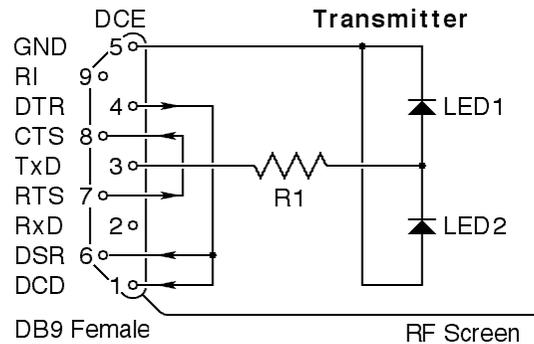
LED1 and LED2 – Red LEDs with non-diffusing package with maximum current ratings of 20 milliamps, a nominal forward voltage drop of 2.2 volts, and a maximum reverse voltage greater than 3 volts. Panasonic LN28RCPP or LN28CPP should work. The non-diffusing package lowers the minimum operating voltage while making alignment between the transmitter's LEDs and the receiver's photodetectors somewhat critical.
