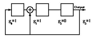
Period, in bits, is 2<sup>n</sup>-1 for an n bit register, *but only if the taps are in the right places!*
