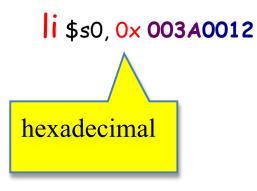
means "load the 32-bit constant into register \$s0." Internally it is translated into
