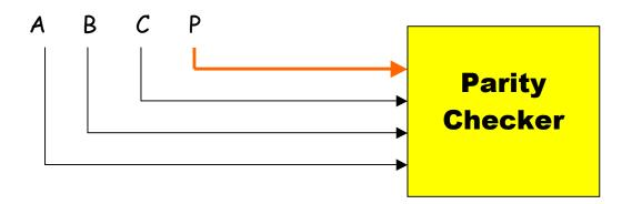
The parity-bit generator generates a P so that the number of 1's in the transmitted data is odd (or even). The **parity checker** checks this in the received data. How will you design (1) a parity-bit generator, and (2) a parity checker?
