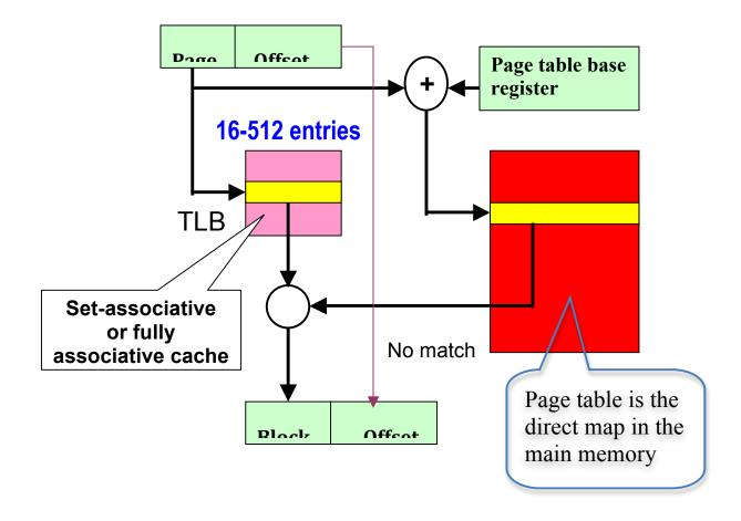
**TLB** is a **set-associative cache** that holds a partial page table. In case of a TLB hit, the block number is obtained from the TLB (fast mode). Otherwise (i.e. for TLB miss), the block number is obtained from the direct map of the page table in the main memory, and the TLB is updated.
