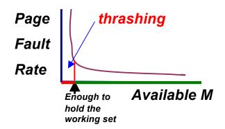
Always allocate enough memory to hold the working set of a program (Working Set Principle)
