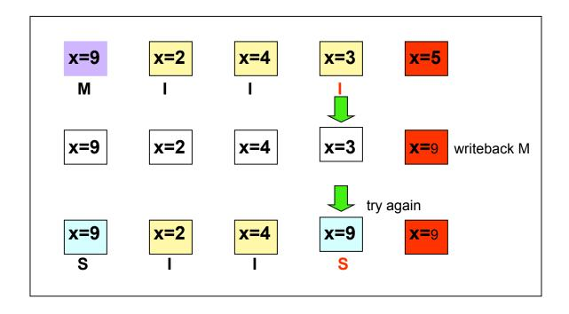
Following the read miss, the holder of the modified copy signals the initiator to try again. Meanwhile, it seizes the bus, and write the updated copy into the main memory.
