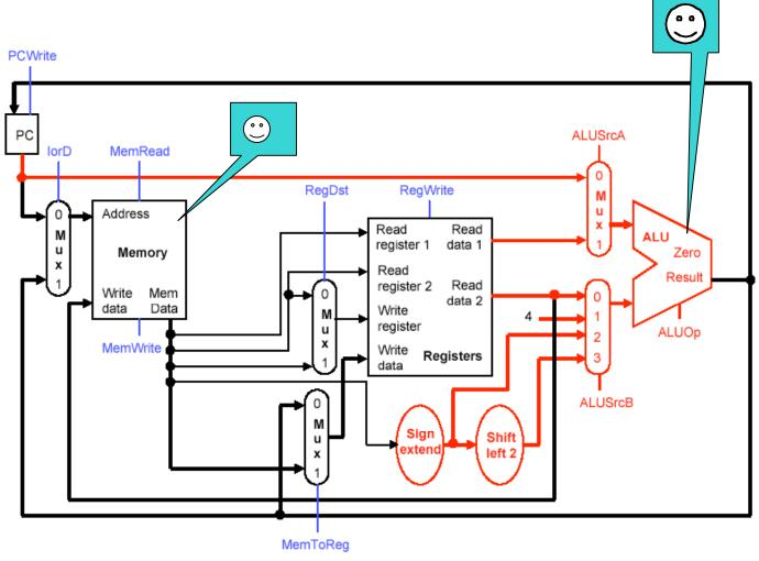
Note that we have *eliminated two adders*, and used only *one memory unit* (so it is Princeton architecture) that contains both instructions and data. It is **not essential to have a single memory** unit, but it shows an alternative design of the datapath.
