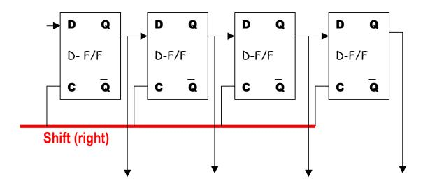
With each clock pulse on the shift line, data moves one place to the right.
