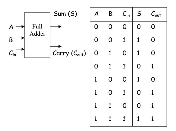
$S = A \oplus B \oplus C_{in}$  $C_{out} = A.B + B.C_{in} + A.C_{in}$
