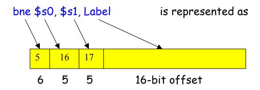
Current PC + (4 \* offset) determines the branch target Label This is called PC-relative addressing.
