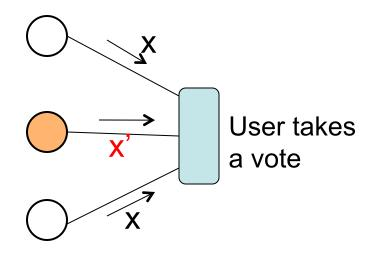
*N-modular redundancy* masks up to m failures, when N = 2m + 1
