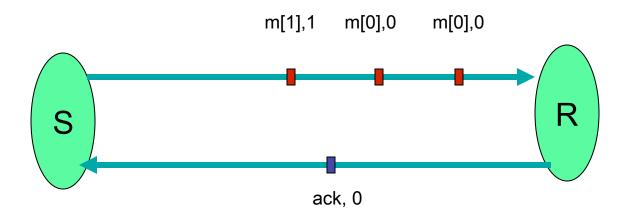
ABP is a *link layer protocol*. Works on **FIFO channels only**. Guarantees reliable message delivery with a **1-bit sequence number** (this is the **t**raditional version with window size = 1). Study how this works.
