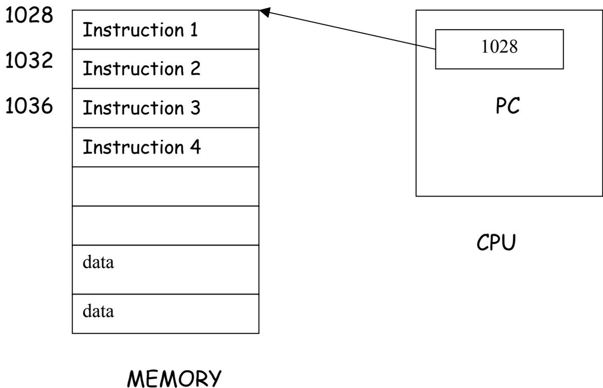
Ordinarily, PC is incremented by 4 after each instruction is executed. A branch instruction **alters the flow of control** by modifying the PC.
