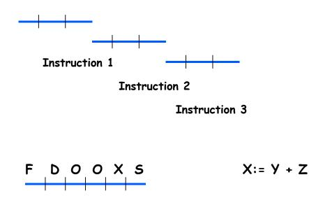
Instruction cycle with six phases: Fetch, Decode, Op fetch, Op fetch, Execute, Store (result). CPI (Cycles Per Instruction) is an important metric for a processor.
