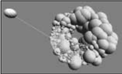
Figure 2: Mesh Sweeping process: As a spherical particle falls towards a torus, the torus mesh is refined in the vicinity of the closest point to the particle, which is indicated by a small sphere, and is connected to the particle by a line.
