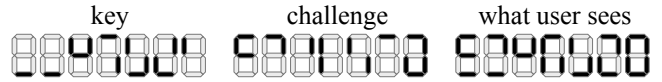
Figure 1: An example of key, challenge and combined frames for an SVAP authentication round.
