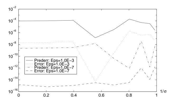
Fig. 7. Predicted and actual errors along the radial line  $\theta=0$  for an exterior Dirichlet problem on an ellipse
