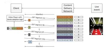
Fig. 1. Architecture of adaptive video streaming for a large-scale live event
