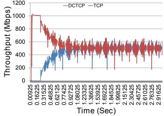
Fig. 2. Throughput of one long-lived DCTCP and TCP flow under a Drop-Tail queue. The bottleneck capacity was 1 Gbps.
