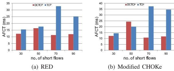
Fig. 7. The figure shows the AFCT of DCTCP and TCP flows under the incast scenario with RED and modified CHOKe.  $min_{th}$  was set to 70.
