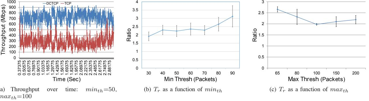
Fig. 4. The figure shows the performance of long-lived DCTCP and TCP flows when the bottleneck link uses RED. (a) Shows the throughput of flows over time for  $min_{th} = 50$  and  $max_{th} = 100$ , (b) shows  $T_r$  as a function of  $min_{th}$  while keeping  $max_{th}$  at 100, and (c) shows  $T_r$  as a function of  $min_{th}$  while keeping  $max_{th}$  at 45.
