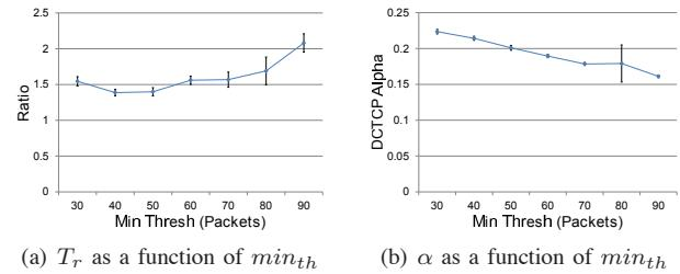
Fig. 6. The figure shows the performance of a single long-lived DCTCP and TCP flow under CHOKe with  $m = 7$  and ECN enabled. (a) and (b) show  $T_r$  and DCTCP  $\alpha$  as a function of  $min_{th}$ , respectively.
