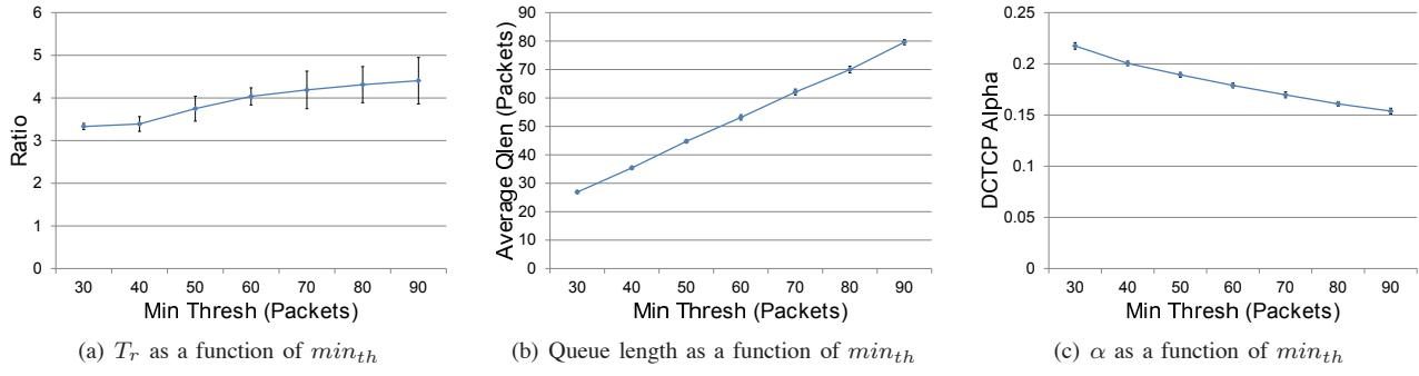
Fig. 5. The figure shows the performance a single long-lived DCTCP and TCP flow under CHOKe with ECN. (a), (b), and (c) show  $T_r$ , average queue length, and  $\alpha$  as a function of  $min_{th}$ , respectively.
