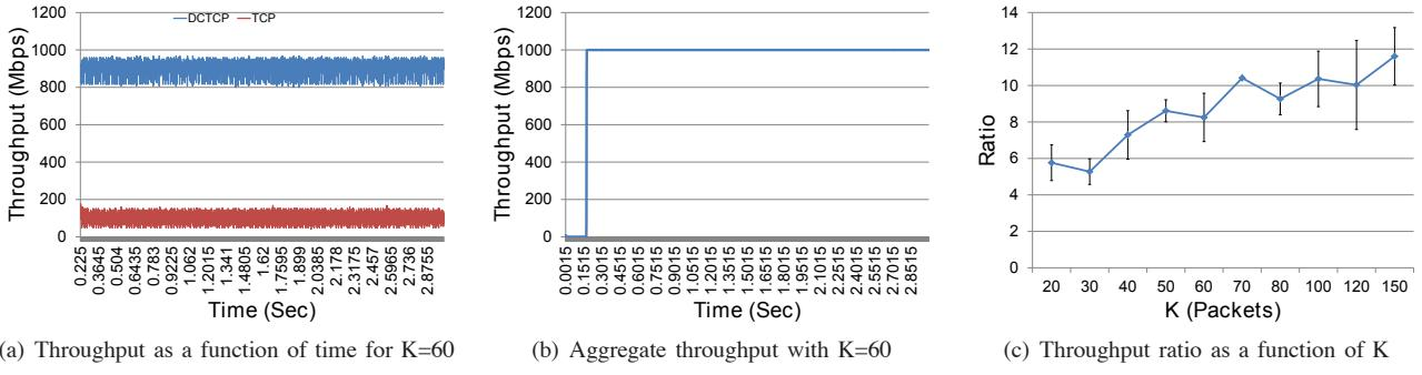
Fig. 3. The figure shows the performance of long-lived DCTCP and TCP flows when the bottleneck link uses the DCTCP AQM. (a) Shows the throughput of flows over time, (b) shows the aggregate throughput of flows, and (c) shows the throughput ratio  $T_r$  as a function of  $K$ .
