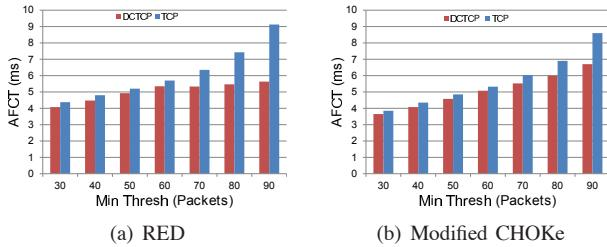
Fig. 8. The figure shows the AFCT of DCTCP and TCP flows under the non-incast scenario with RED and modified CHOKe. The offered load of short flows is set to 20% of bottleneck capacity.
