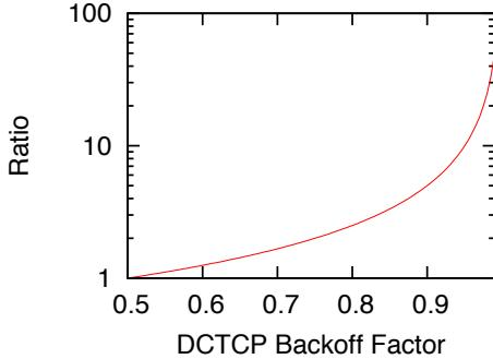
Fig. 1. Throughput ratio  $T_r$  (DCTCP/TCP) with various  $\beta_{dctcp}$  values.
